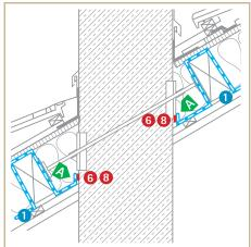
Sub-and-top installation Sealing to concrete chimney
