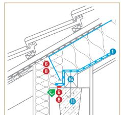
Knee wall sealing, sub-and-top with continuous rafter
