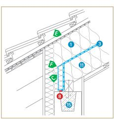
Sealing at knee wall with continuous rafters
