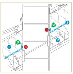
Sealing to plastered chimney
