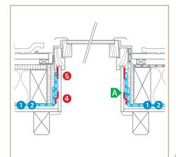
Sealing at skylights – Longitudinal section
