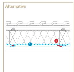
Sticking membrane overlaps perpendicular to rafter
