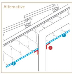
Pipe feed-through with adhesive tape
