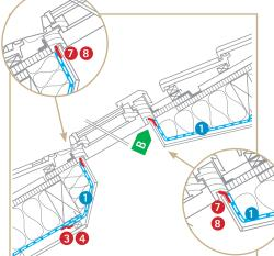
Sealing at skylights Transverse cross-section
