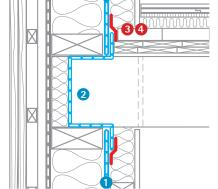
Penetration Beams or angular components
