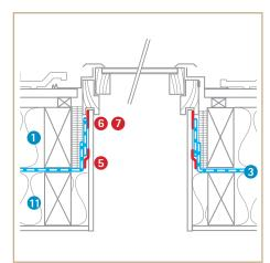
Sealing at skylights – Longitudinal section
