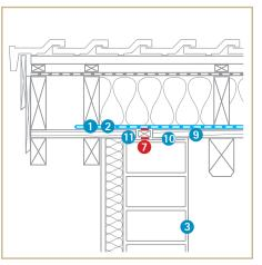
Sealing at bargeboard with interrupted boarding
