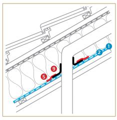
Pipe feed-through for sub-and-top and tub-shaped
