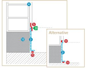
Sealing at ground or ceiling slab with interior insulation
