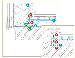
Sealing to solid ceiling or ground slab
