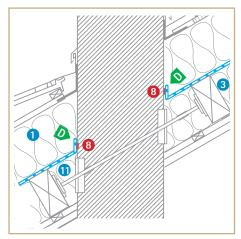
Sealing to concrete chimney
