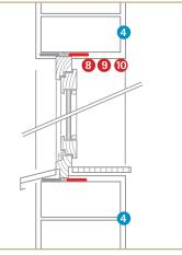
Sealing at windows, at the side of the frame, masonry wall
