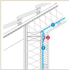
Sealing at knee wall for timber structures
