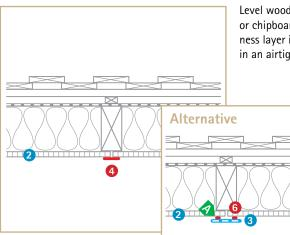
Level wood-based panels such as OSB, plywood or chipboard panels can be used as an airtightness layer if joints and connections are sealed in an airtight manner.
